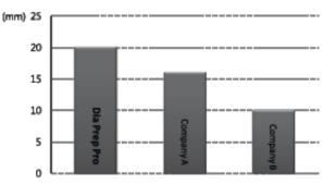
This comparison test was done according to ISO6876 regulations (setting time & condition as per DiaDent R&D laboratory)
